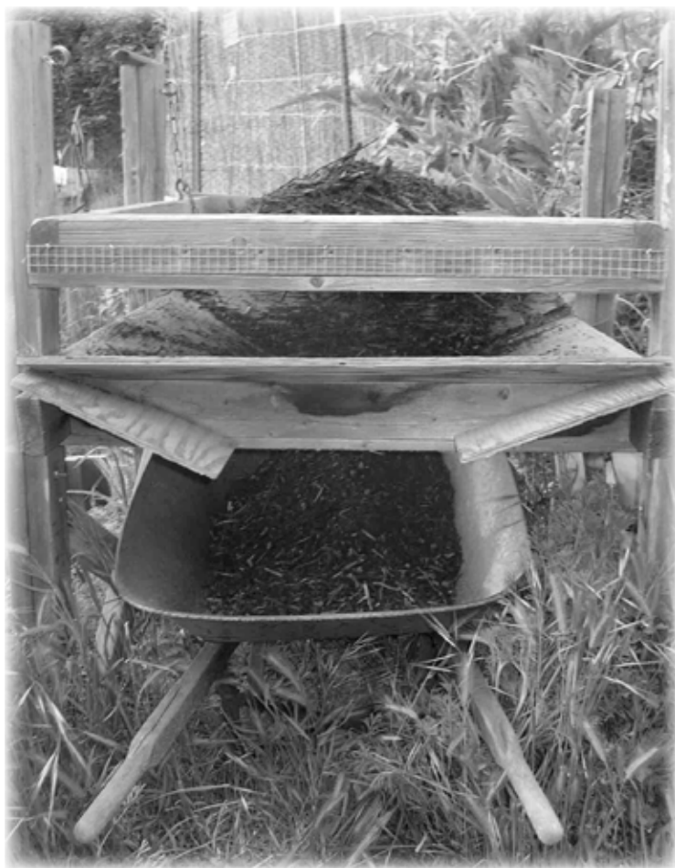
A compost sifter helps remove un-decomposed roughage.
